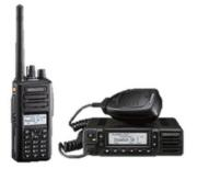
NX-3000 Series radios can be configured to simultaneously support FM Analogue + one digital access protocol, but offers the flexibility for users to switch between either of the two digital protocols easily and cost effectively:
